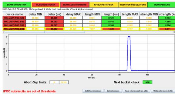
Figure 8: IQC MKI panel showing the MKI waveform of magnet D which had a flashover and had a length of about  $2\mu\text{s}$  only instead of the required  $8\mu\text{s}$ .
