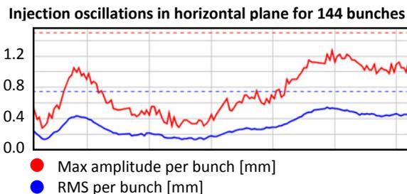
Figure 7: Injection oscillations amplitudes in the horizontal plane for 144 bunches for beam 2. A bunch-by-bunch variation of more than 1 mm was discovered. [01:28:57 25/9-2011]
