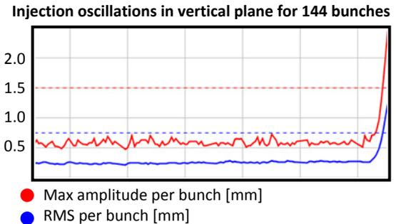
Figure 6: Injection oscillations in the vertical plane for 144 bunches. The last bunches had larger oscillation amplitudes due to too short kicker waveform. [23:21:38 20/6-2011]
