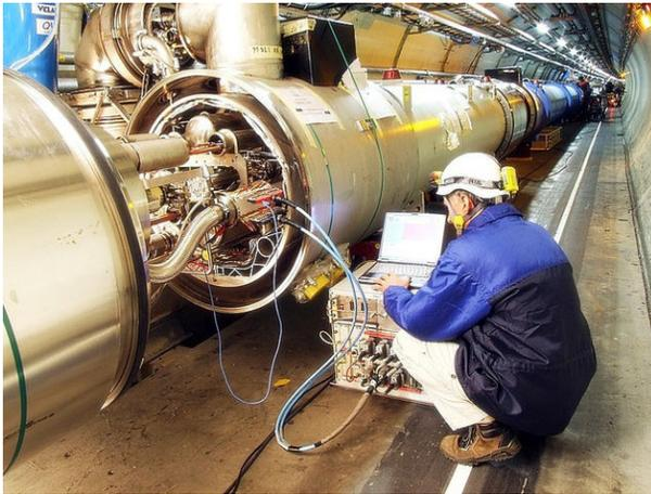
Figure 2: High Voltage qualification in the LHC tunnel.
