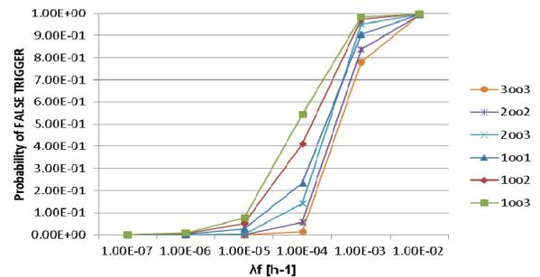
Figure 4: Probability of *False trigger* against  $\lambda f$  between  $1E-7 h^{-1}$  and  $1E-2 h^{-1}$ .
