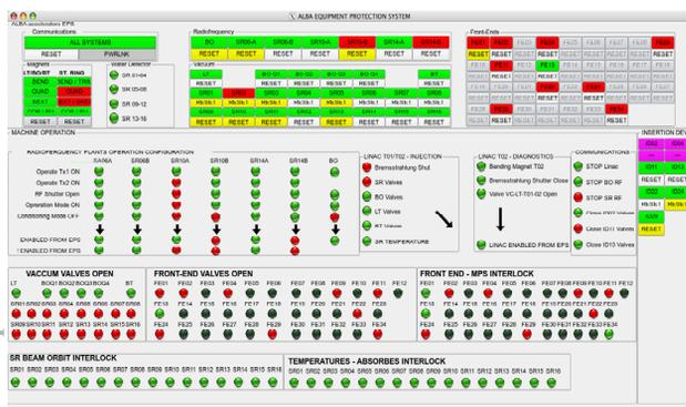
Figure 3: The main EPS GUI for the Machine.
