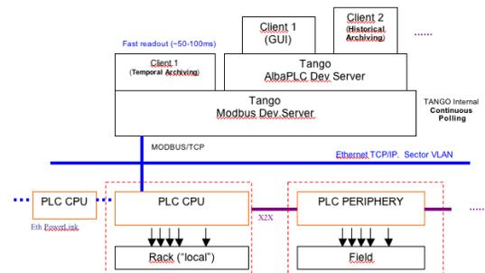
Figure 1: Architecture of the EPS PLC System.
