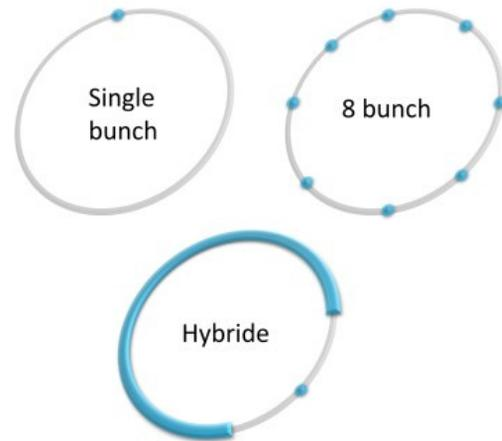
Figure 2: Hybrid, single and 8 bunch filling mode.
