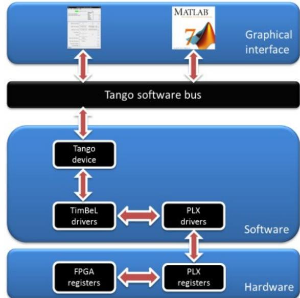
Figure 5: Software architecture.
