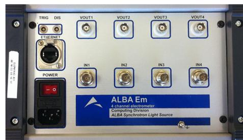
Figure 2: Low resolution electrometer rear panel.
