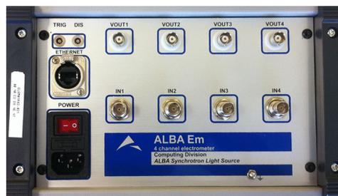
Figure 2: Low resolution electrometer rear panel.
