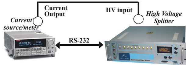
Figure 4: High Voltage Splitter calibration.
