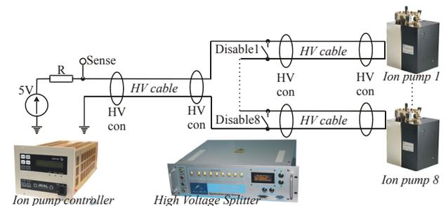
Figure 6: Cable Interlock diagram for one ion pump controller, HVS and 8 pumps.
