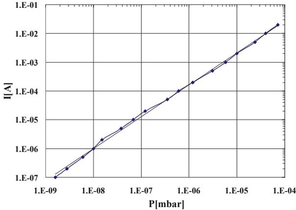
Figure 2: 25lps noble diode ion pump, Uconst=7kV.
