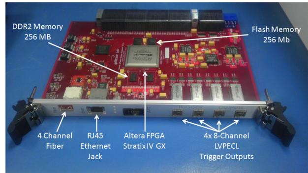
Figure 4: GTP Prototype.
