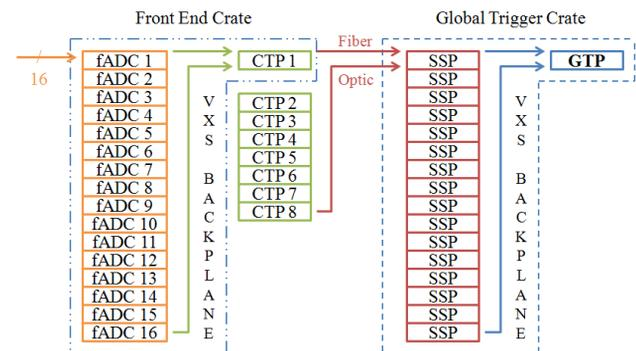
Figure 1: Level 1 Trigger System Data Flow.
