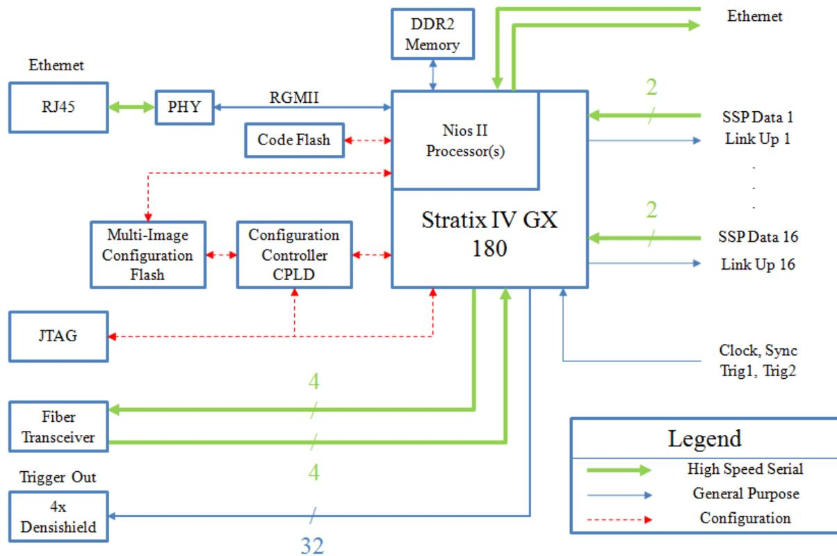
Figure 3: Simplified Global Trigger Processor Hardware Block Diagram.
