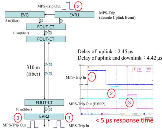
Figure 6: Timing measurement of uplink and downlink with 310 m fiber and three stages of fan-out concentrator.
