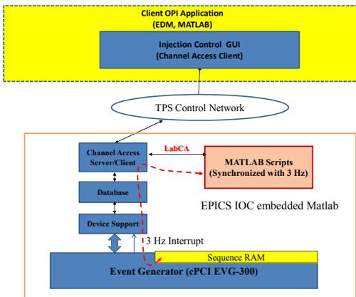
Figure 7: Block diagram of proposed timing sequence control.
