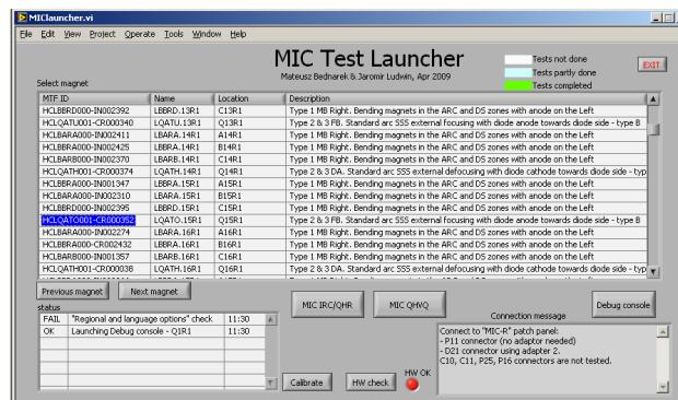
Figure 2: MIC Test Launcher, with list of available magnets to be tested and information about hardware connections that are required to perform tests on a selected magnet.
