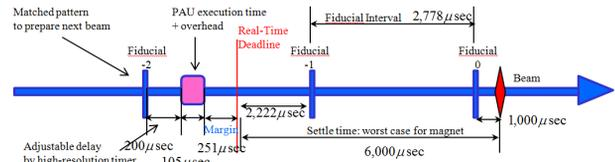
Figure 5: Performance Measurement and Real-Time Deadline.
