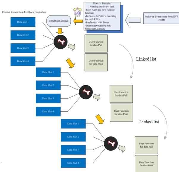
Figure 2: PAU processing for the Multiple Muxes.
