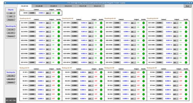
Figure 3: The operation interface of storage ring dipole, quadrupole and sextupole magnet power supplies.
