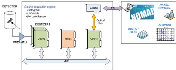
Figure 2: Schematic view of the acquisition engine.
