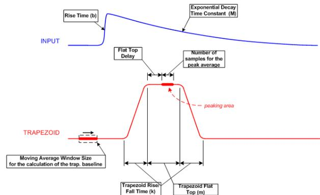
Figure 1: Trapezoidal filter with the relevant parameters.
