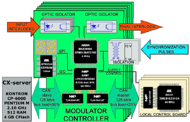
Figure 2: Modulator Controller and Local Control Boards.
