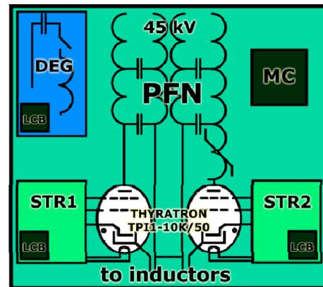
Figure 1: Modulator structure.
