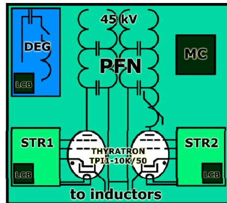
Figure 1: Modulator structure.
