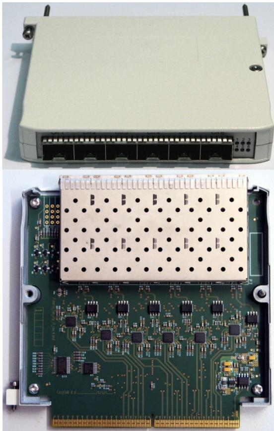
Figure 3: FlexRIO Adapter Module with 6 generic optical
