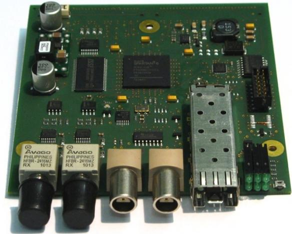
Figure 4: FPGA based front end device board.
