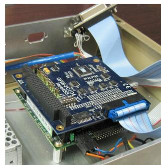
Figure 2: GPIB-PC/104-XL Module Stacked on the PC/104 IOC.
