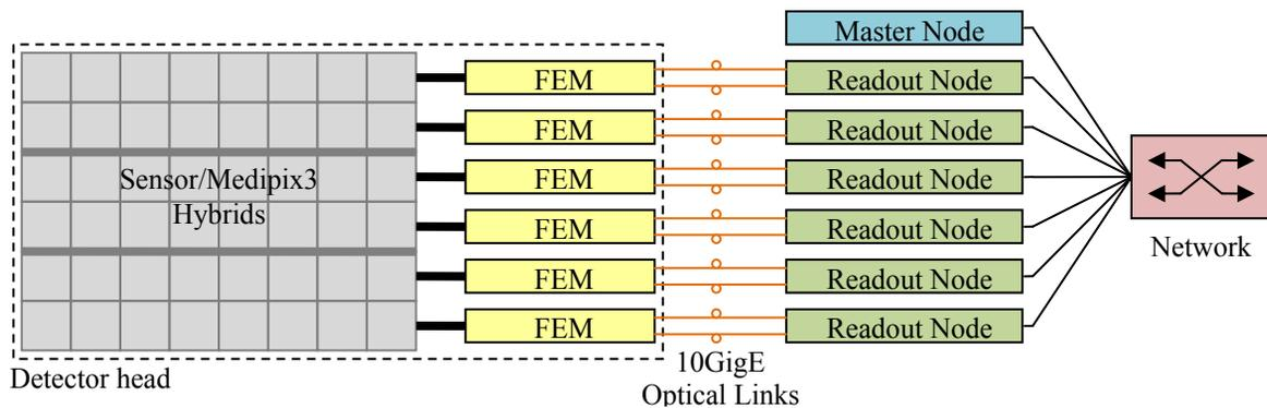
Figure 1: Hardware architecture.
