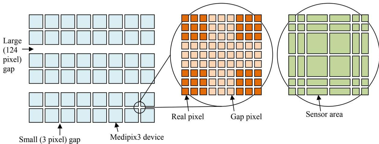
Figure 5. Medipix3 device layout and gap details.
