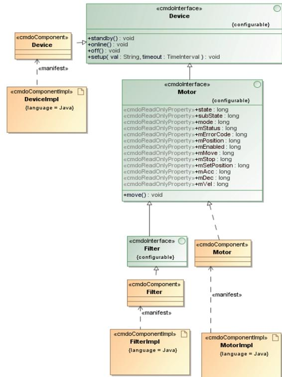
Figure 3&lt;Specifications for motors in the prototype0
