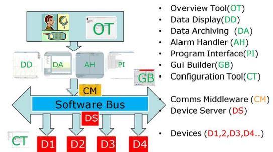
Figure 1: SCADA requirements.
