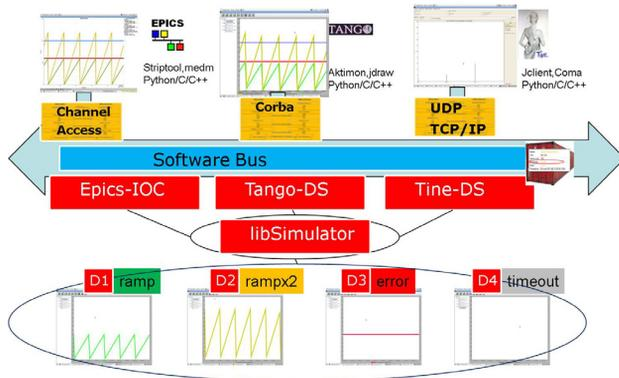
Figure 7: libSimulator test setup.
