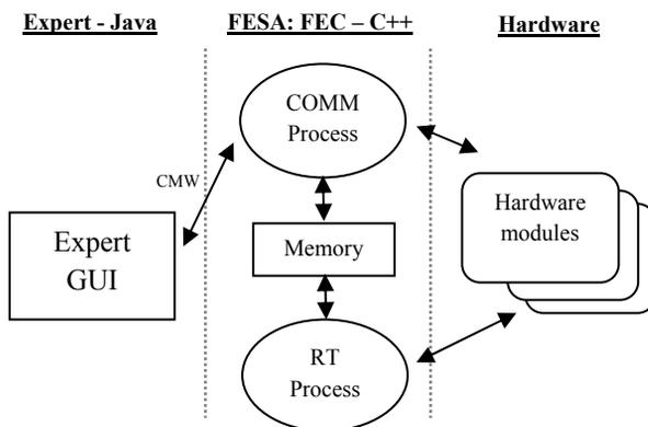
Figure 1: BE Front-End Software Architecture (FESA).
