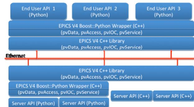
Figure 3: Software Structure by Wrapping V4 Modules.
