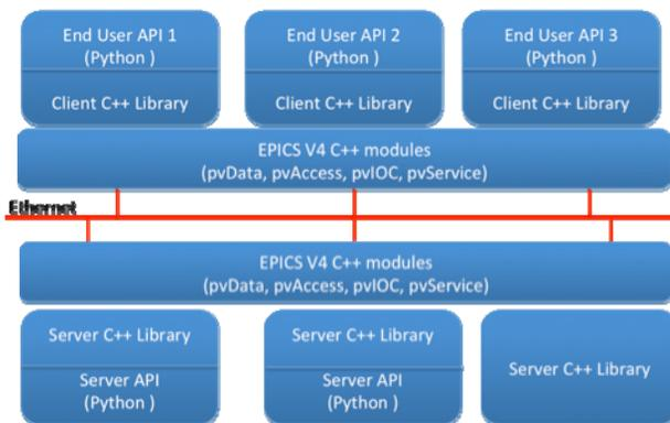
Figure 2: Software Structure Using Python/C.
