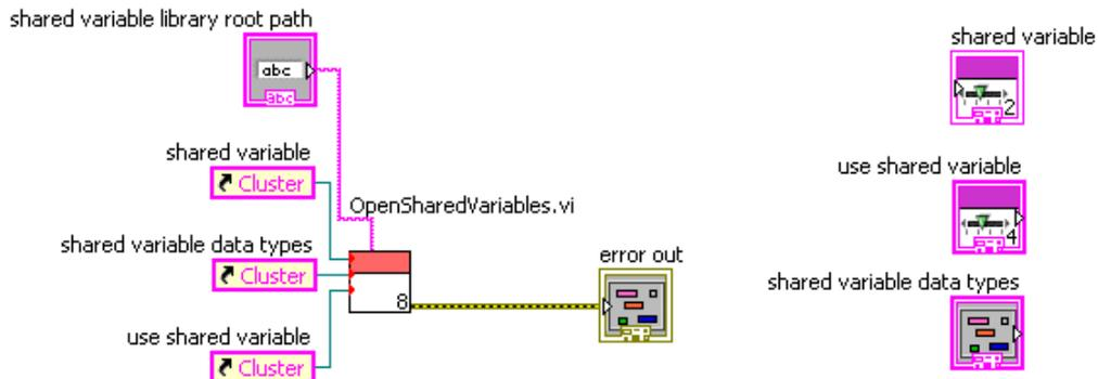
Figure 6: Example of an auto-generated VI that uses the generic VI from Figure 5 for opening shared variables from a specific library.
