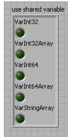
Figure 4: Example of an auto-generated “access cluster”.
