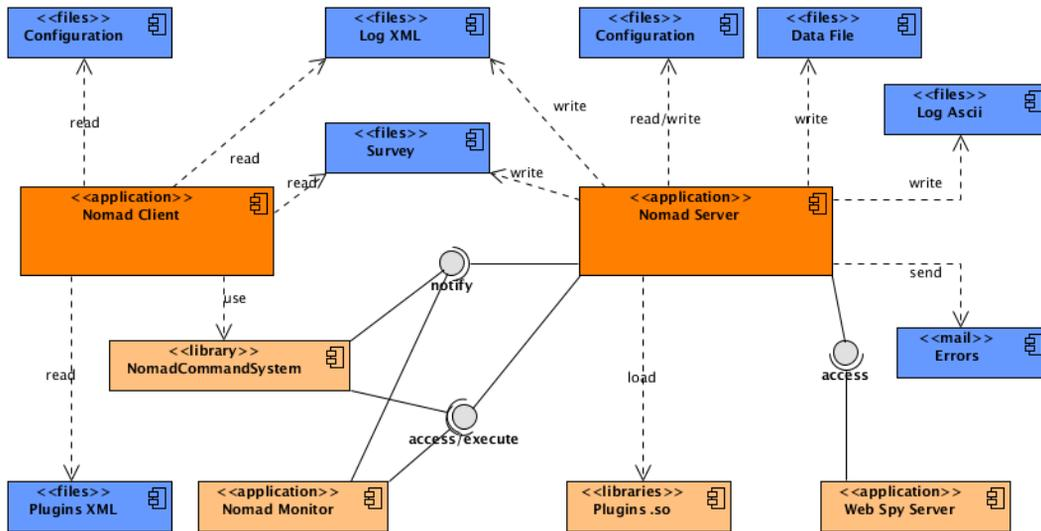
Figure 1: Simplified component diagram for the NOMAD application.
