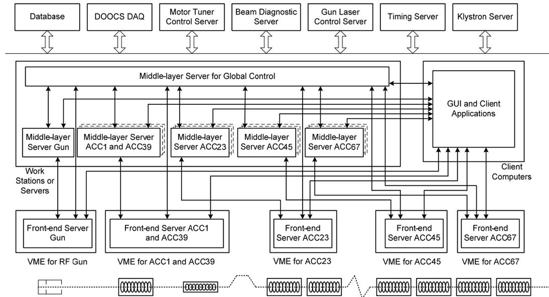
Figure 8: Allocation of the LLRF applications.
