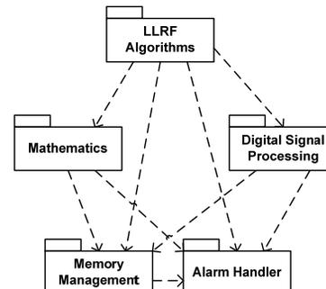
Figure 6: Domain breakdown of the LLRF Algorithm Library.
