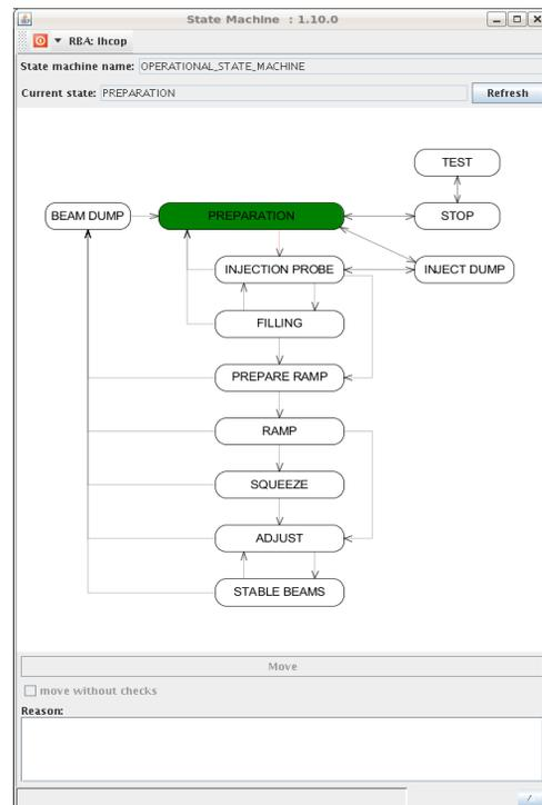
Figure 1: LHC Operational States diagram in SM GUI.
