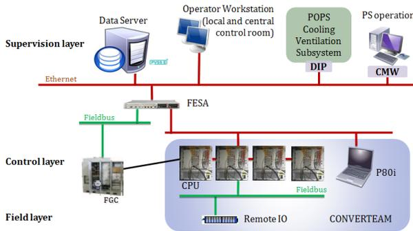
Figure 2: POPS control hardware architecture.
