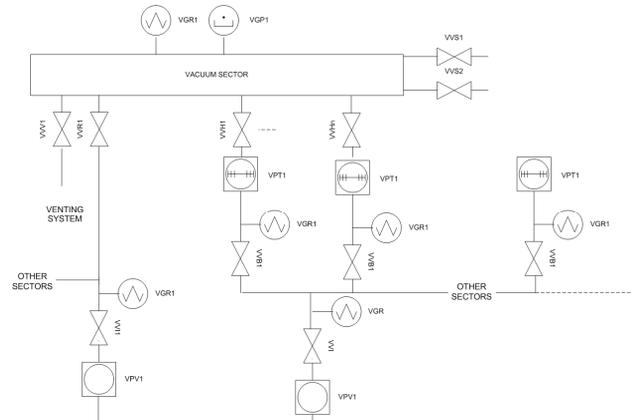
Figure 2: Plant schema of an ISOLDE vacuum sector.
