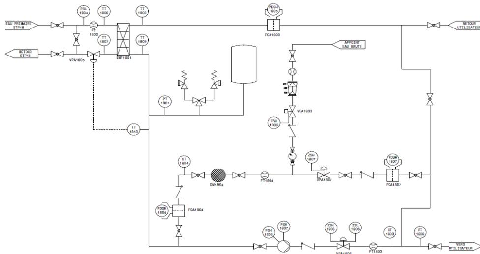
Figure 4: Plant schema of the STP18 cooling plant.
