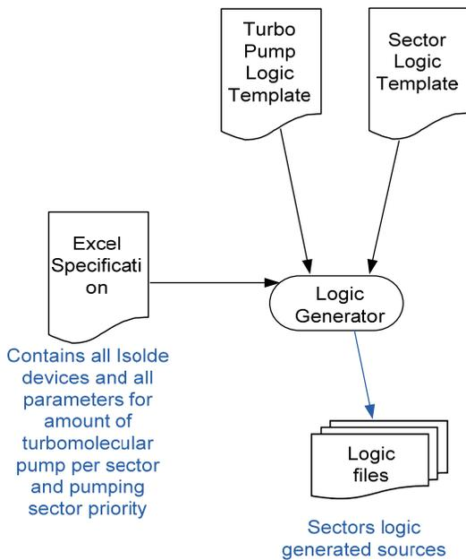
Figure 3: Principle of automatic logic generation.
