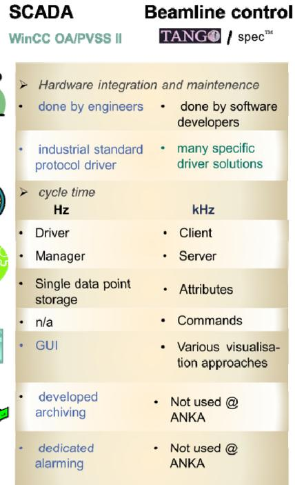
Figure 1: Comparison chart of basic features of WinCC OA and Tango based beamline control. Key benefits of the SCADA and TANGO used at ANKA are marked blue.
