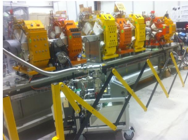
Figure 1: Typical NSLS-II girder assembly
