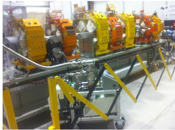
Figure 1: Typical NSLS-II girder assembly
