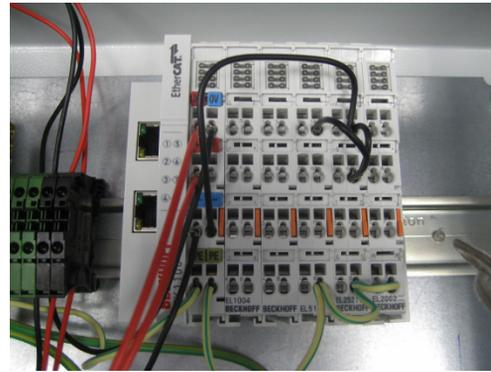
Figure 3: PS control modules before wiring.
