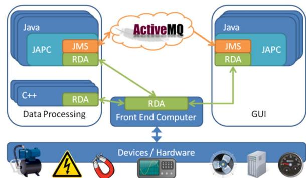
Figure 1: Usage of the Control System Middleware.
