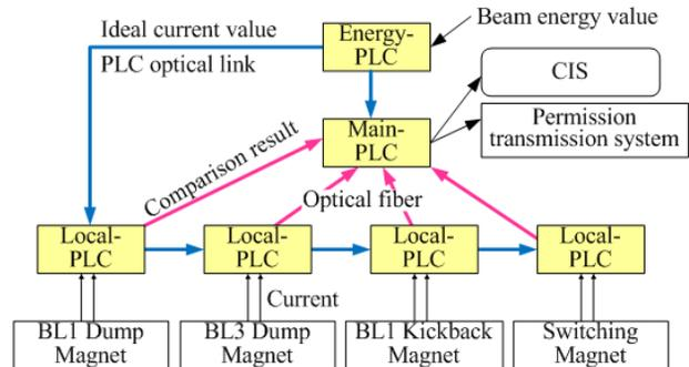
Figure 3: Schematic of the beam route interlock system.
