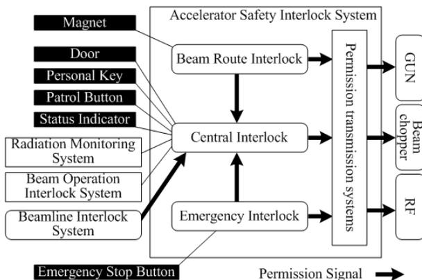
Figure 2: Schematic of the radiation safety interlock system.
