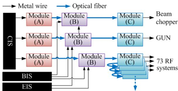
Figure 4: Schematic of the permission transmission system.
