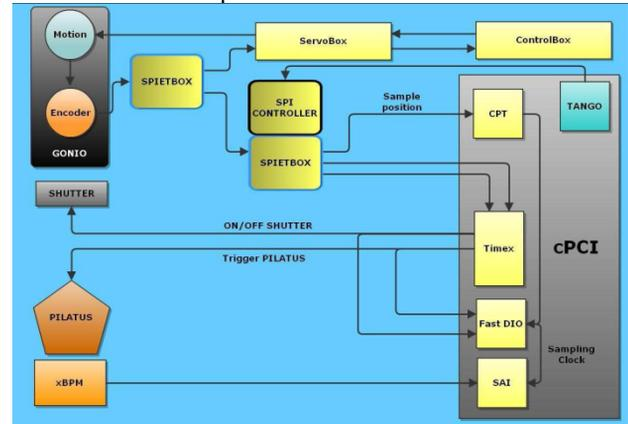
Figure 5: Architecture for PX1 acquisition with Pilatus.
