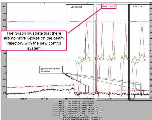
Figure 4: Acquisition showing the difference between old and new control system of HU256 undulators.
