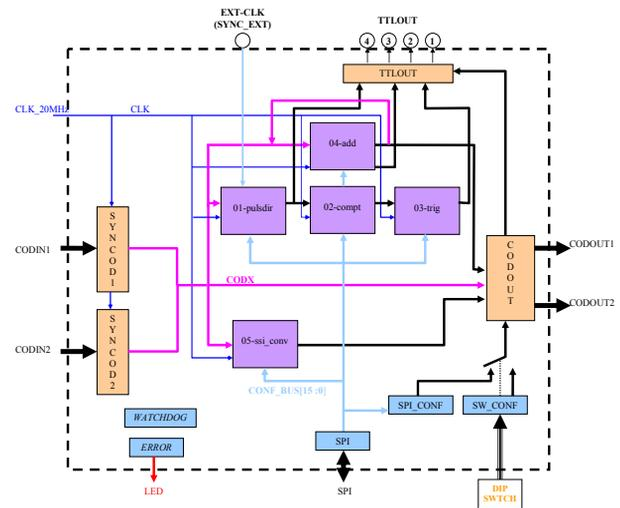
Figure 2: FPGA architecture of protocol conversion for encoders.
