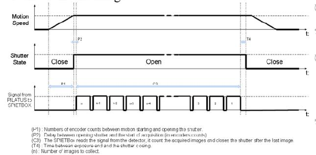
Figure 6: Timing of the most use triggering mode.
