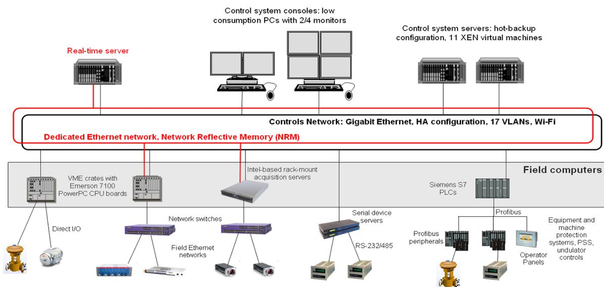
Figure 2: Architecture of the FERMI@Elettra control system.
