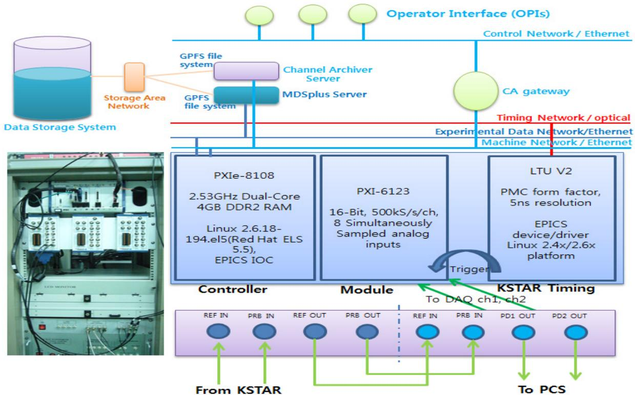
Figure 1: Configuration of MMWI DAQ System and network connections to the infrastructure of the KSTAR control system.
