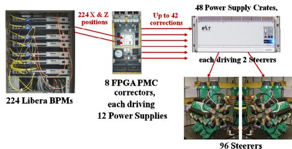
Figure 2: Fast Orbit Feedback System.
