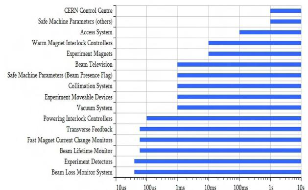
Figure 1: Reaction Times of CERN Interlock systems.<sup>1</sup>
