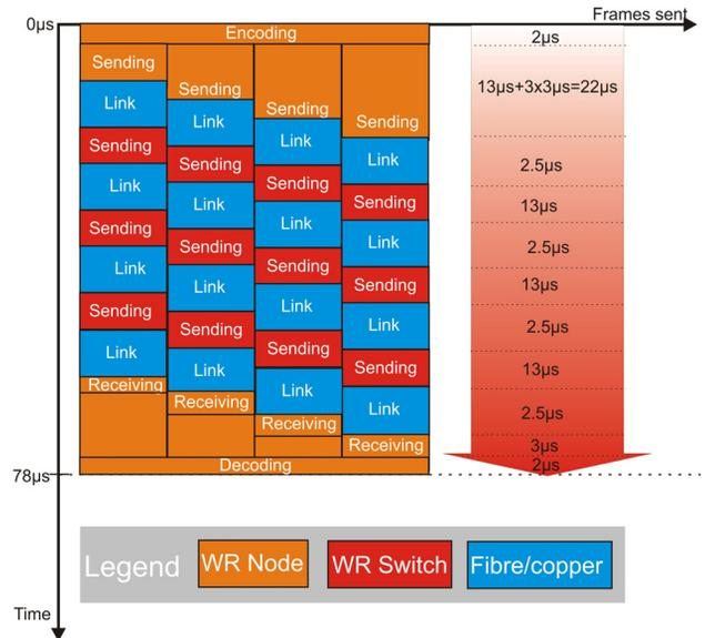
Figure 2: Delivery Delay of Control Message using cut-trough<sup>2</sup>
