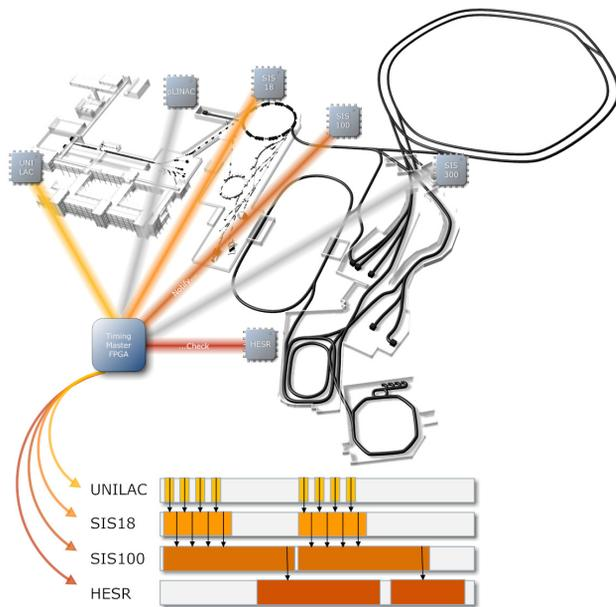
Figure 3: Machine sequences in a production chain.
