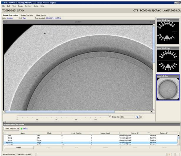
Figure 4: Control panel for x-ray imaging engine.
