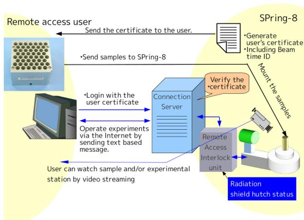
Figure 1: A schematic of the SPring-8 remote experiment system.
