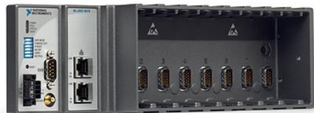
Figure 1: The National Instruments cRIO 9074 [2].
