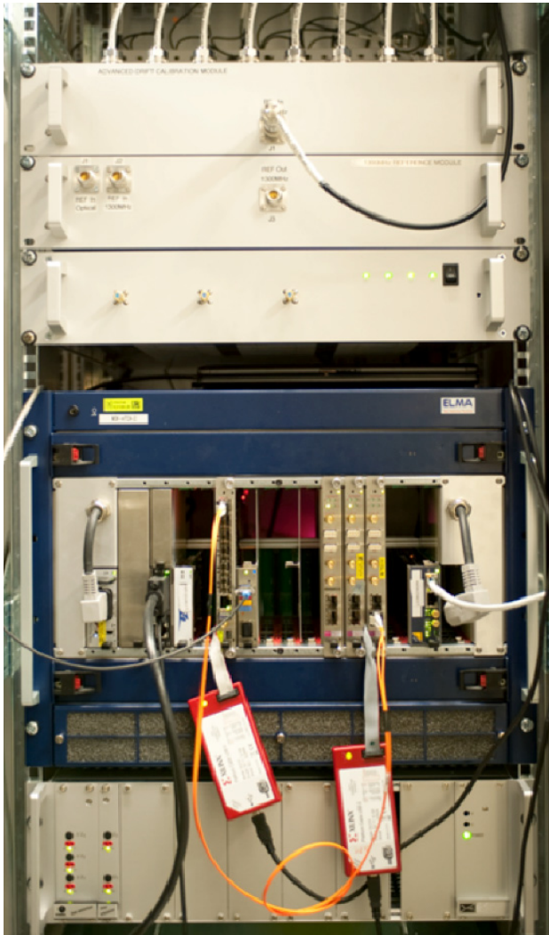
Figure 2: The rack with the blue MicroTCA crate controls 8 superconducting cavities of one cryo module in FLASH.
