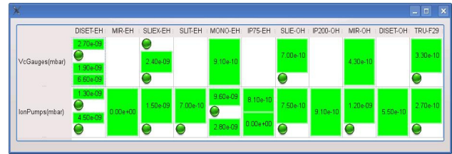
Figure 5: Labels from cabling are used to group in grids the experimental equipment pressures.
