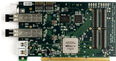
Figure 3: CERN Read-Out Receiver Card (PCI-X slot) with 2 Destination Interface Units.
