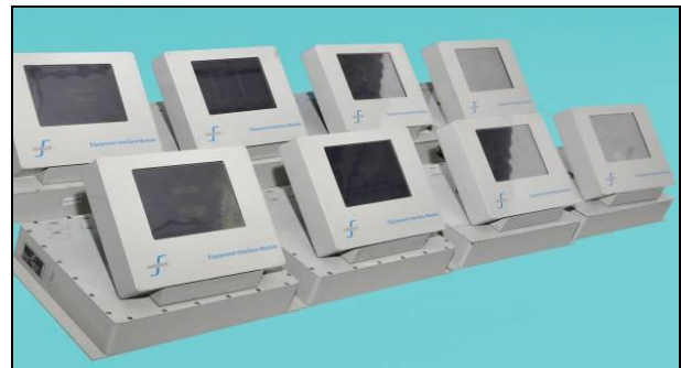
Figure 3: Snapshot of Equipment Interface Modules (EIMs).
