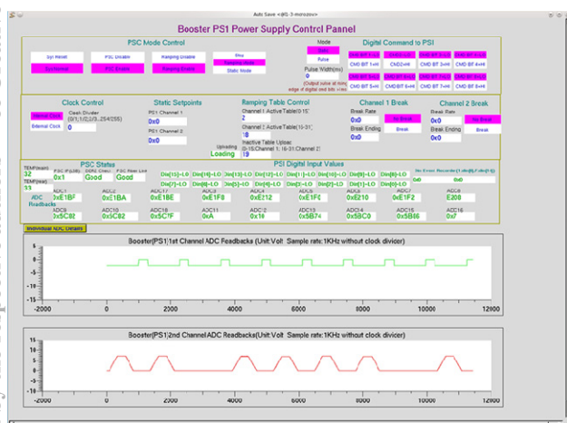
Figure 3: EDM screen for testing of PSC/PSI.
