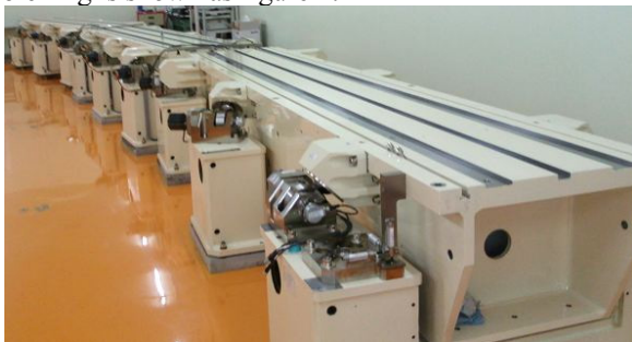
Figure 1: One twenty-fourth of the whole ring consists of three girders.
