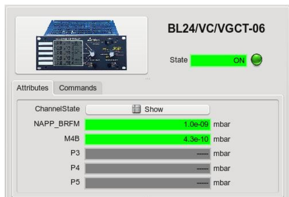
Figure 4: Names of vacuum gauge ports are labelled with the tag of the device connected to them.
