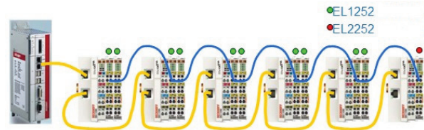
Figure 8: Time resolution test. EL1252 module sends a pulse and all EL2252 measure this pulse and takes a timestamp. The difference of these timestamp is the time resolution of the system.
