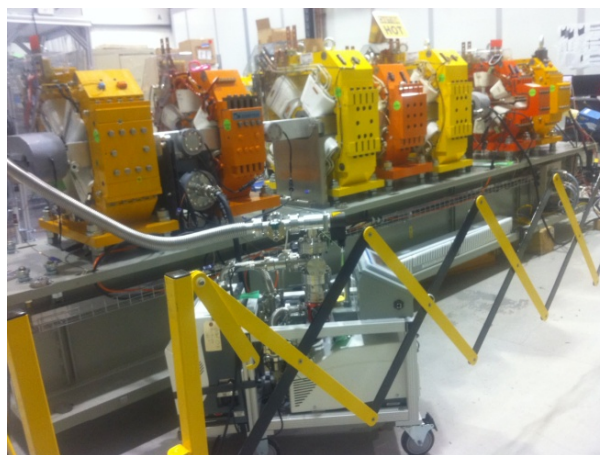
Figure 1: Typical NSLS-II girder assembly
