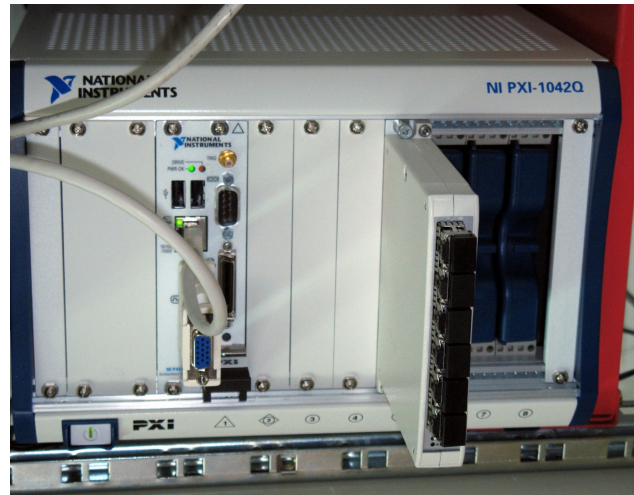
Figure 3: PCC test setup with 1 FlexRIO FPGA board and mounted 6-way optical real-time link adapter.
