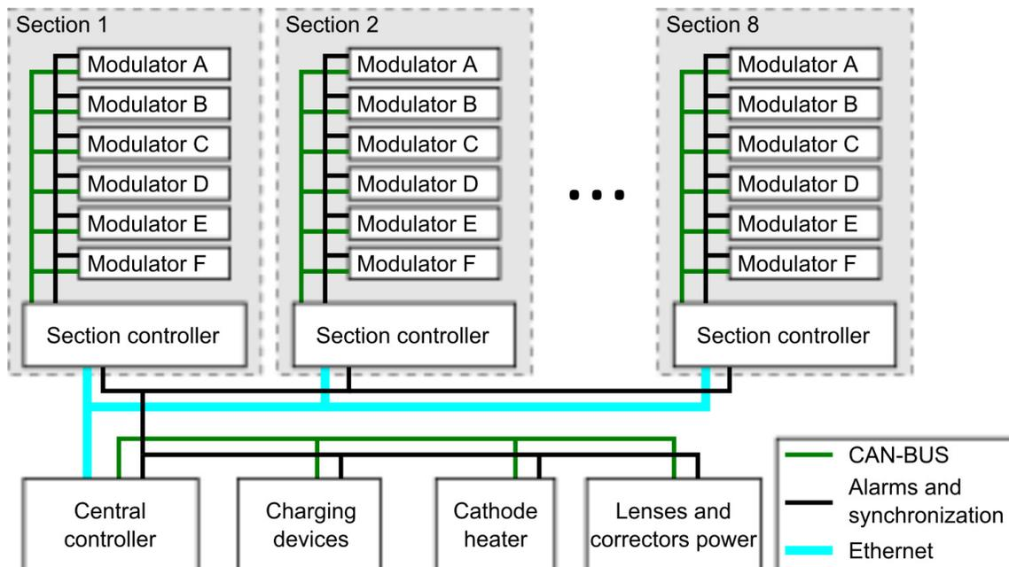
Figure 2: The structure of LIA control system.
