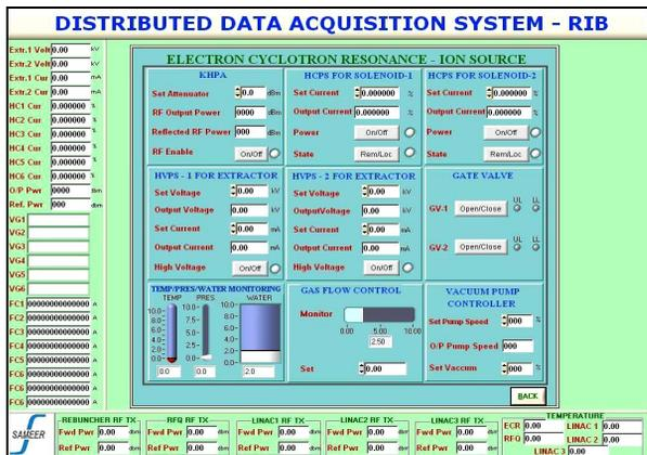
Figure 6: A typical GUI for ECR-IS Subsystem.
