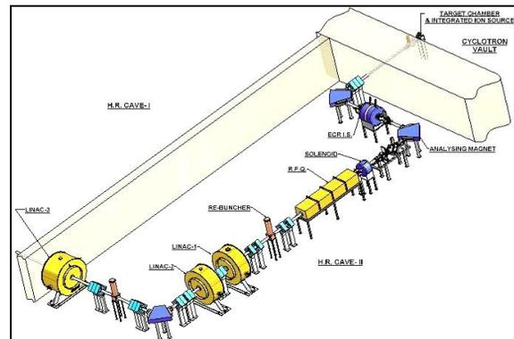
Figure 1: Layout of RIB facility (up to LINAC-3).
