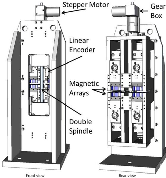
Figure 5: Motion control components of the phase shifter.
