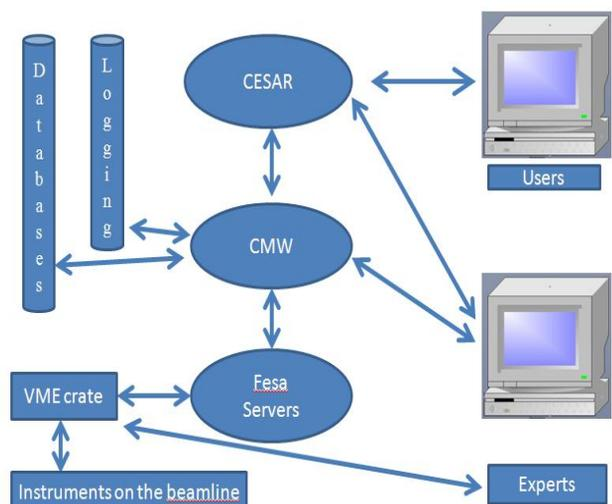
Figure 2: The three tier Software structure used.
