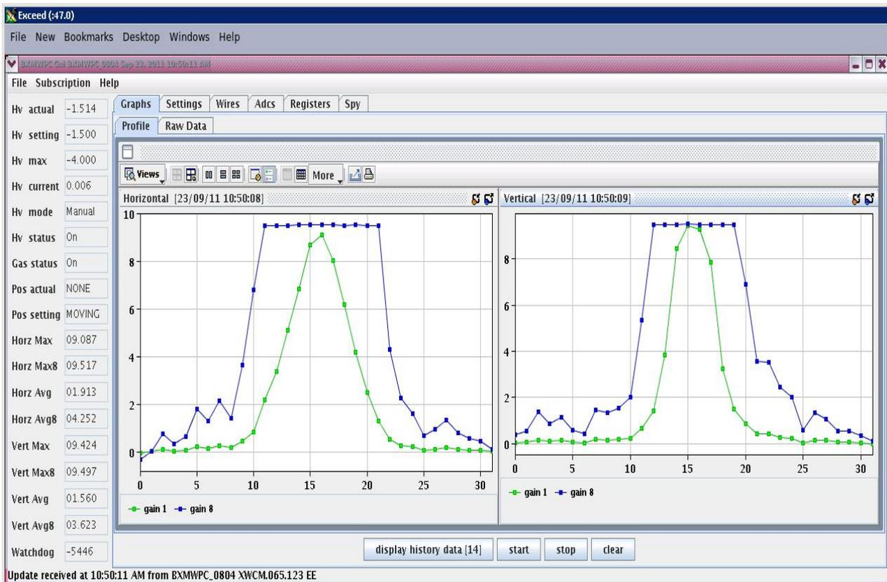
Figure 3: Example of an expert GUI, this one is for the control of an Analog wire chamber.
