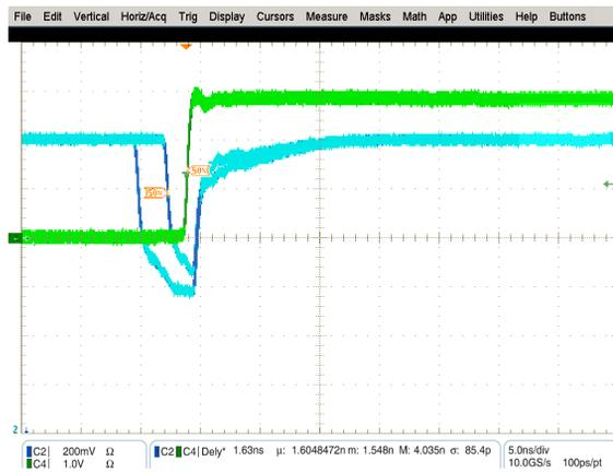
Figure 3: Delay is 600ps use CML output.
