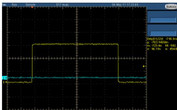
Figure 4: The blue signal is the input signal of interlock, its level is low when there are no interlocks. The yellow signal is the output of EVR.
