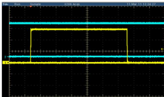
Figure 5: When the blue signal needs to realize the interlock function, it becomes high level, and the yellow signal is shutdown it just becomes low level.
