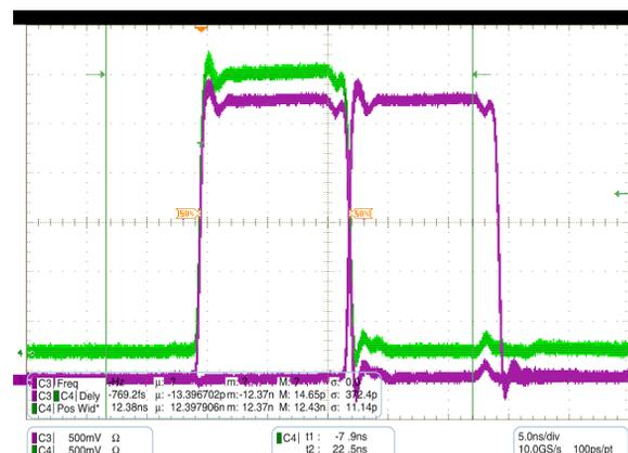
Figure 2: Delay is 12ns use common output.
