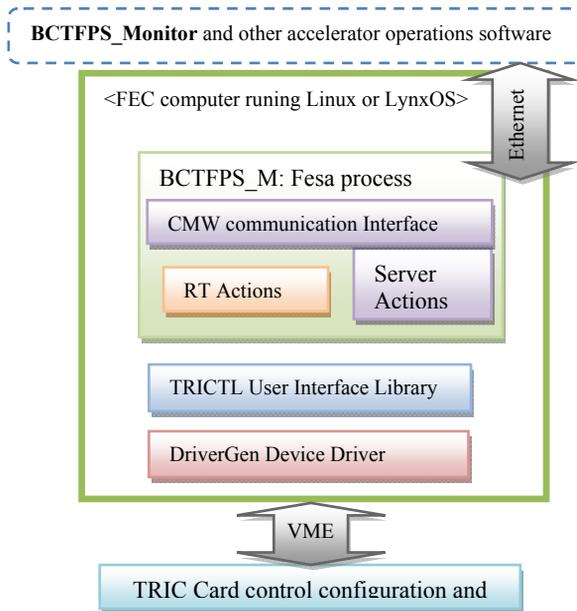
Figure 3: Software structure.
