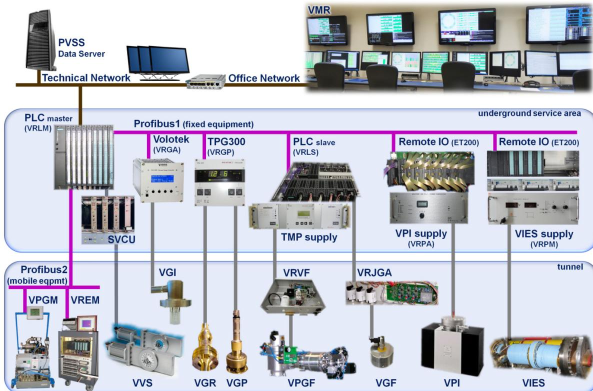
Figure 1: LHC vacuum controls architecture.
