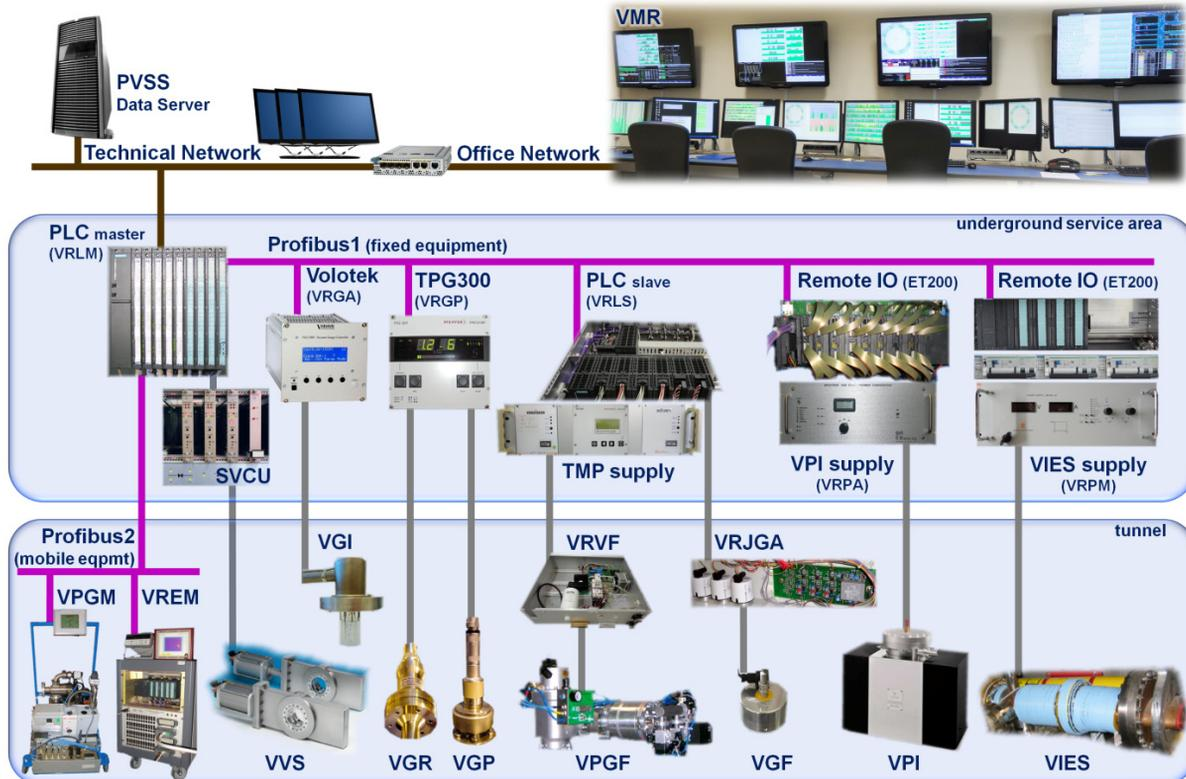
Figure 1: LHC vacuum controls architecture.
