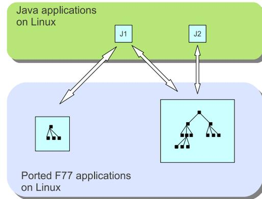
Figure 5: *uv*-architecture for data object exchange between Fortran and Java applications.
