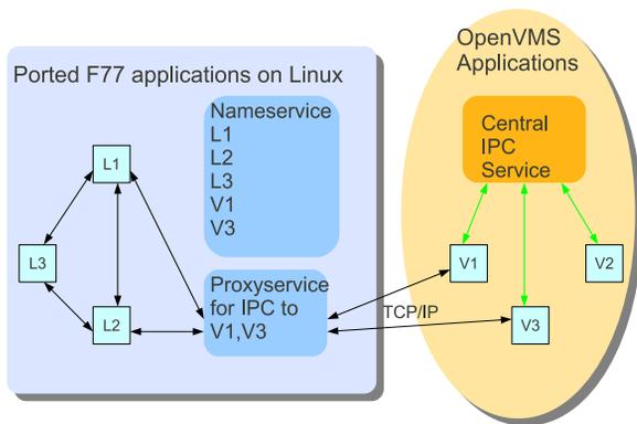
Figure 3: Binary data exchange between Linux and OpenVMS.
