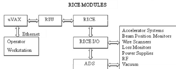
Figure 2: Block Diagram of the RICE System.
