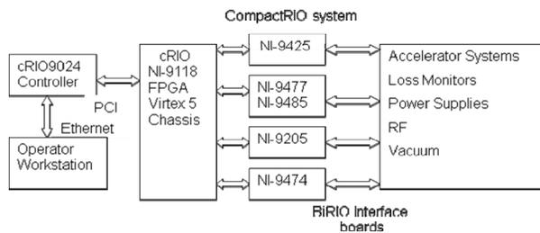
Figure 4: Block Diagram of the cRIO System.
