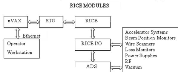
Figure 2: Block Diagram of the RICE System.
