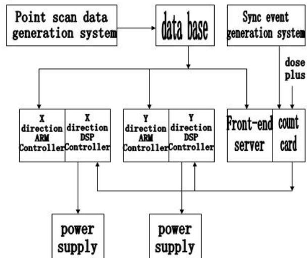
Figure 2: System components.
